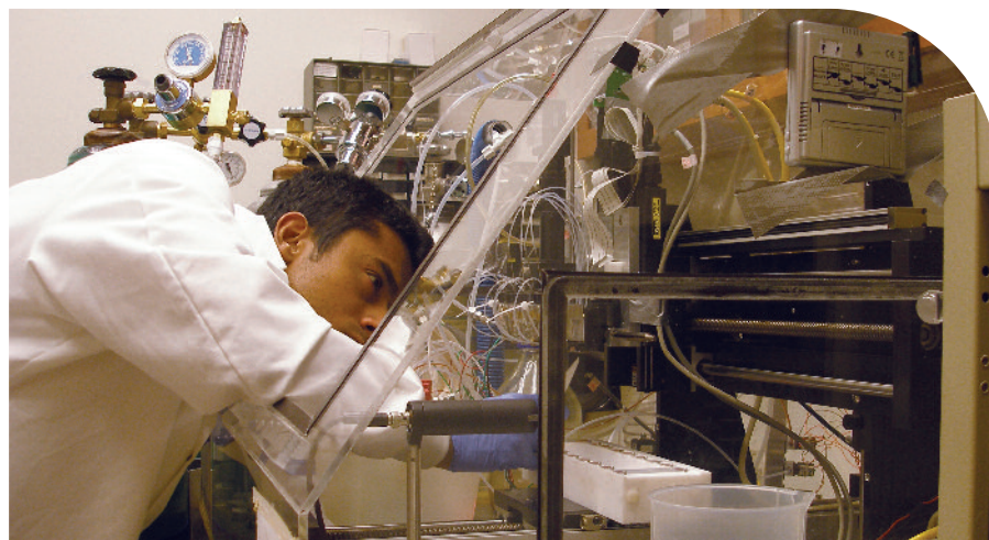
Graduate student Ali Saaem tinkers with the prototype inkjet DNA synthesizer.
